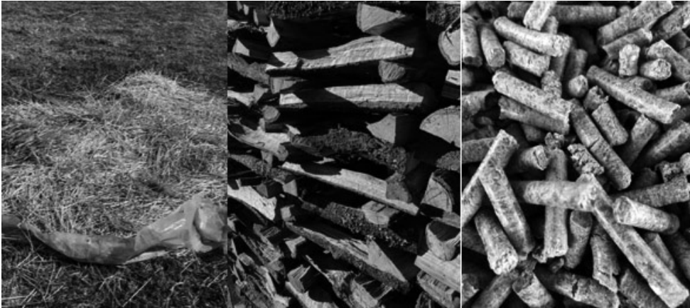
Figure 1. Types of solid biofuels, on the right pine sawdust pellets, in the center white oak firewood, and on the left agricultural pruning stubble
