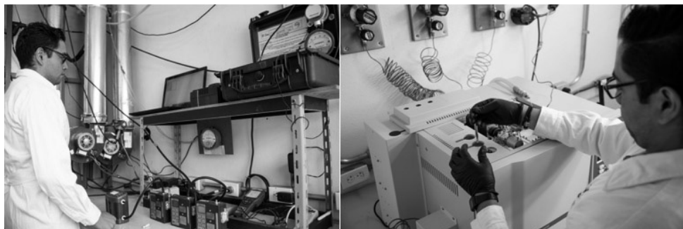
Figure 2. Equipment for measuring emissions. On the right a gas chromatograph and on the left a set of gas flow analyzers.
